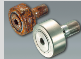
Uncoated (left) and Corrotect-coated track roller (right) following a salt spray test
